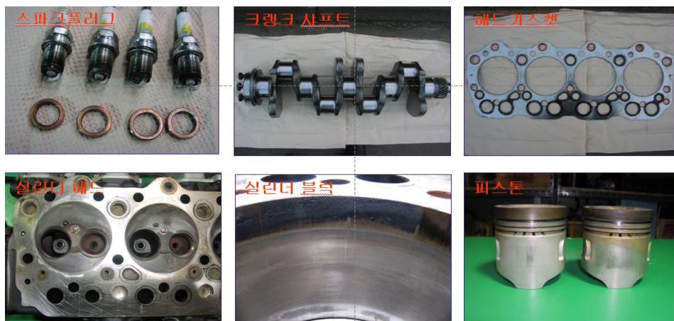
< Fig. 9 > Components verification after vehicle durability test of 50,000Km
