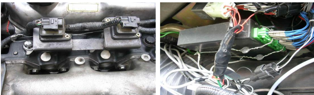
< Fig. 10 > Components to be sealed (Cylinder head / ECU )
