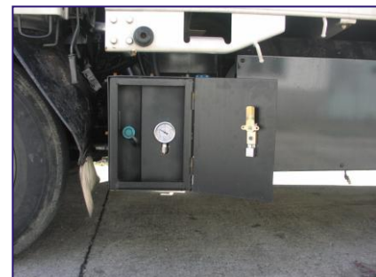
< Fig 4 > Installation of CNG cylinder and fuel module
