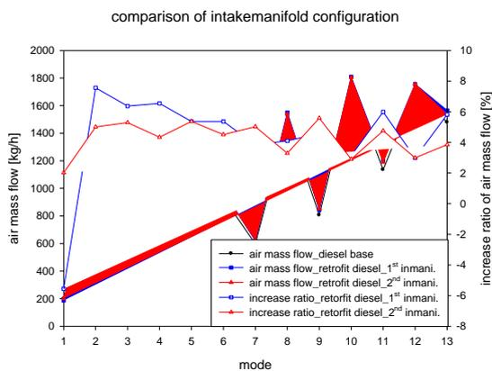
Fig. 11 Variation of air mass flow for deference of intake manifold configuration
