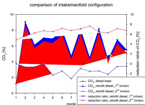
Fig. 12 Variation of CO2 concentration for deference of intake manifold configuration
