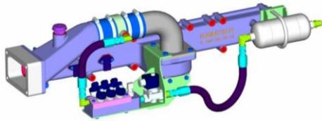
Fig. 4 Configuration of 2<sup>nd</sup> retrofitted intake manifold
