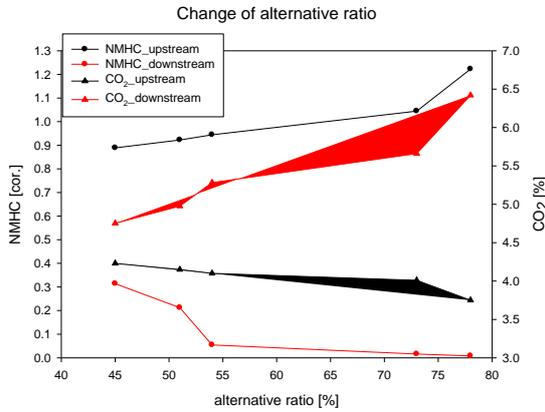
Fig. 7 Variation of harmful emissions for change of alternative ratio; 1600rpm, 25% load
