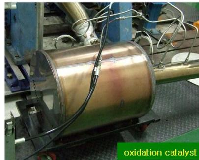
Fig. 6 Oxidation catalyst of dual fuel engine
