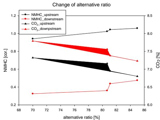
Fig. 8 Variation of harmful emissions for change of alternative ratio; 1600rpm, full load
