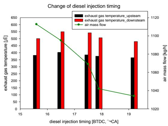
Fig. 10 Variation of exhaust gas temperature and air mass flow for change of diesel injection timing; 1600rpm 50% load
