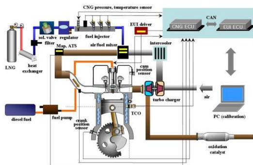
Fig. 2 Schematic of dual fuel system
