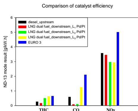
Fig. 13 Comparison of catalyst efficiency for  $P_d/P_t$  ratio;  $L_1 > L_2 > L_3$
