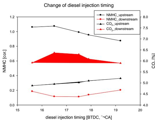
Fig. 9 Variation of harmful emissions for change of diesel injection timing; 1600rpm, 50% load
