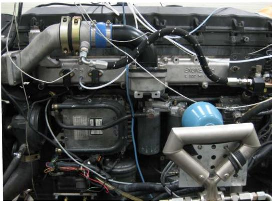
Fig. 1 Dual fuel engine
