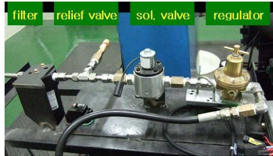
Fig. 5 LNG supply parts
