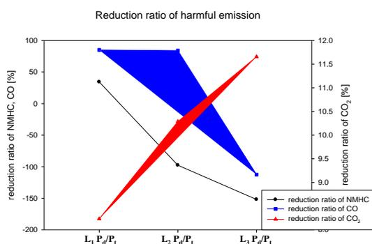
Fig.14 Comparison of reduction ratio for  $P_d/P_t$  ratio;  $L_1 > L_2 > L_3$
