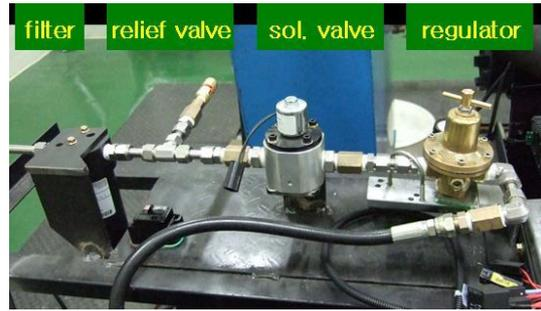
Fig. 5 LNG supply parts
