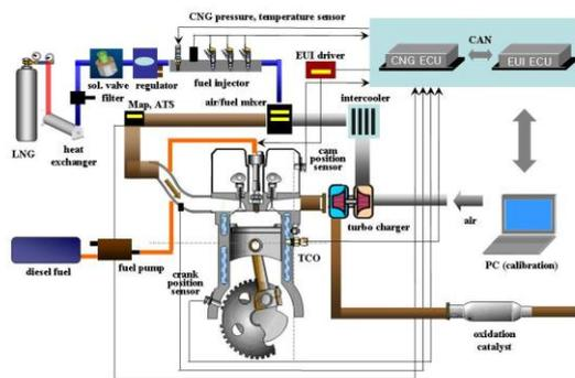
Fig. 2 Schematic of dual fuel system
